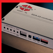
The SDA-03: the intelligent heart of the automatic sliding door.
